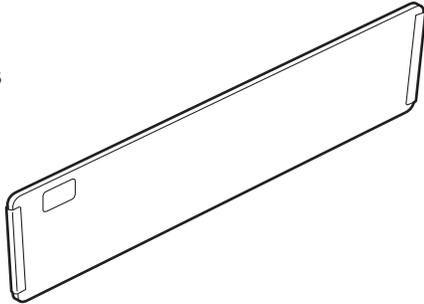
1. Open the tailgate, then open the in-bed trunk lid. Insert the trunk dividers into the six grooves (three grooves in the front and three grooves in the rear). Install each trunk divider with the arrow pointing toward the front of the vehicle.
