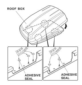
2. Using isopropyl alcohol on a shop towel, clean the four brackets B where the small pads will attach. Remove the adhesive backing from the small pads, and attach them to brackets B.
