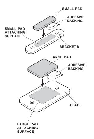
3. Using isopropyl alcohol on a shop towel, clean the four plates where the large pads will attach. Remove the adhesive backing from the large pads and attach them to the plates.
