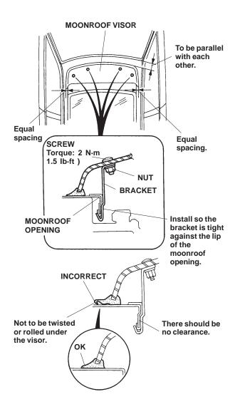
10. Torque the screws to 2 N·m (1.5 lb-ft), alternating between sides. To prevent damage to the resin nuts, do not over-tighten the screws.
