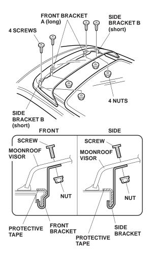
While holding the visor in place, install the four screws, four nuts, and four brackets A and B with the end of each bracket hooked to the lip of the moonroof opening. Do not tighten the screws yet.  Position the moonroof visor with equal spacing on all sides. Check that the rubber seal is not twisted or rolled under the visor.
