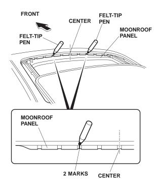
Locate the panel folding line on the right side of the moonroof opening. Measure 87 mm to the front of the vehicle, and make a mark on the roof in two places. Repeat on the other side of the moonroof opening.
