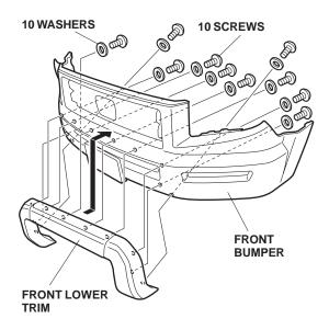
Reinstall the front bumper. Check that all retaining tabs and clips are installed properly without play or rattle.
