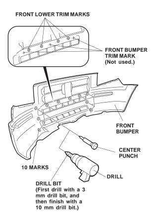
Position the front lower trim on the front bumper, and install the ten screws and ten washers.
