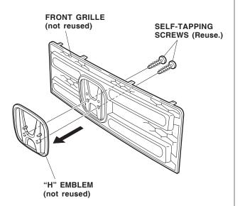
4. Slide the pins from the new "H" emblem into the holes in the new front grille, and install the two self-tapping screws you just removed.
