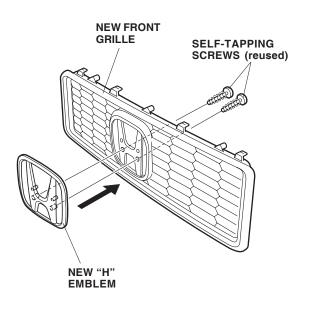
5. Position the new front grille on the front bumper, and install it with the eight retaining tabs.
