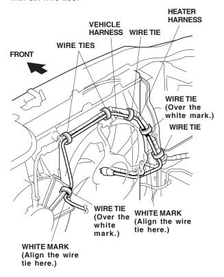
Continue routing the heater harness along the vehicle harness and down to the bumper grille opening. Attach the protective cap to the bumper grille, and plug the heater harness connector into the protective cap.
