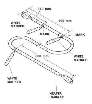
6. Plug the heater harness connector into the engine block heater, and secure the heater harness to the vehicle harness with one wire tie at the white mark.
