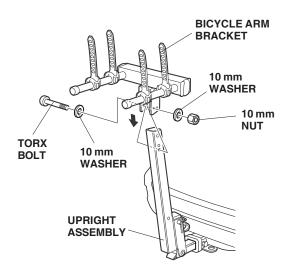
3. Install the torx bolt with two 10 mm washers and the 10 mm nuts. Tighten the torx bolt securely.
