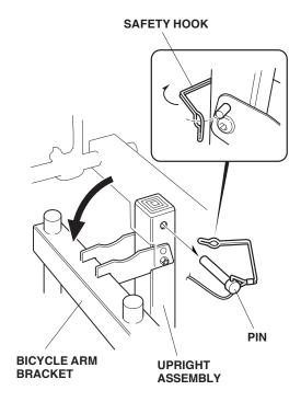
2. Reinstall the pin and safety hook.
