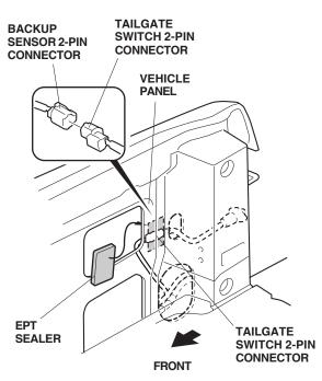
67. Using isopropyl alcohol on a shop towel, clean the areas where the EPT sealer will attach. Secure the backup sensor harness to the vehicle frame with one EPT sealer.
