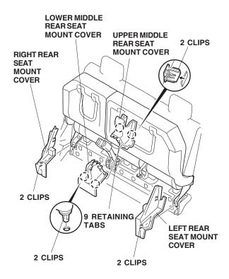
14. Remove the caps from the rear trim panel cover (four retaining tabs for each cover).
