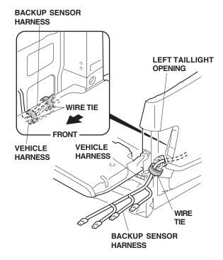
53. Continue routing the backup sensor harness along the rear bumper area, and secure it to the vehicle harness with eight wire ties.
