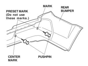
38. While wearing eye protection, drill one 19 mm (¾ in.) hole and one 25 mm (1 in.) hole through the marks on the rear bumper. First drill with a 3 mm bit, then finish with a 19 mm (¾ in.) hole saw and 25 mm (1 in.) hole saw. Remove any burrs from the edges of the holes.
