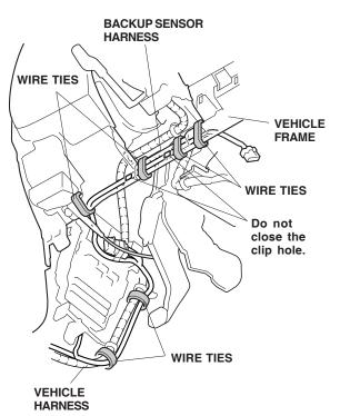
If the vehicle is equipped with a security system, wrap one cushion tape around the backup sensor harness, and secure the backup sensor harness to the security system bracket with the wire tie.
