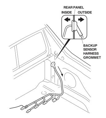
49. Inside the cargo area, route the backup sensor harness along the vehicle harness, and secure the front of the harness to the body with one white wire tie with clip.
