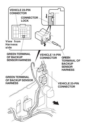
74. Push the green terminal from the backup sensor harness into vehicle 23-pin connector, then reattach the connector lock. Reconnect the vehicle 23-pin and 14-pin connectors. 75. Route the backup sensor harness forward. Secure the backup sensor harness to the vehicle harness with four wire ties and two small wire ties in the area shown.
