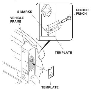
60. While wearing gloves and eye protection, drill a 26 mm hole and four 8 mm holes through each of the marked locations. First drill with a 3 mm drill bit, then finish the center hole with a 26 mm hole saw and the outer holes with an 8 mm drill bit.
