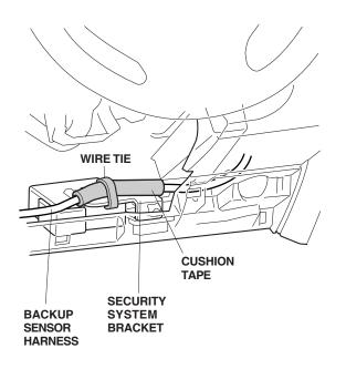
80. Continue routing the backup sensor harness down along the vehicle harness, and secure it to the vehicle harness and frame with three wire ties.
