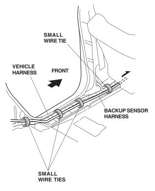
77. Continue routing the backup sensor harness along the vehicle harness, and secure it to the vehicle harness with three small wire ties.
