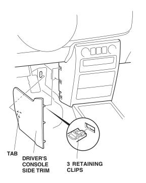
6. Remove the passenger's console side trim (two retaining clips and one tab).
