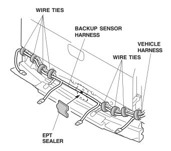
54. Using isopropyl alcohol on a shop towel, clean the area where the EPT sealer will attach. Secure the backup sensor harness to the vehicle panel with one EPT sealer at the green tape.
