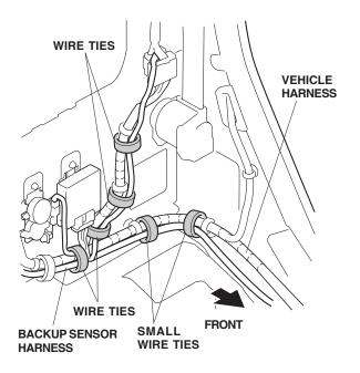
76. Route the backup sensor harness forward along the vehicle harness, and secure the backup sensor harness to the vehicle harness with four small wire ties.
