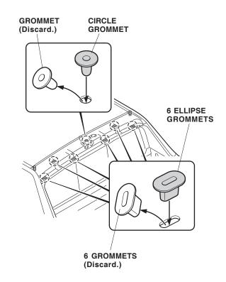
27. On the inside of the rear roof trim, remove and discard the clips, and install the seven new clips to the rear roof trim.
