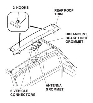
26. Remove and discard the grommets from the roof panel. Install the six ellipse grommets and one circle grommet into the roof panel.
