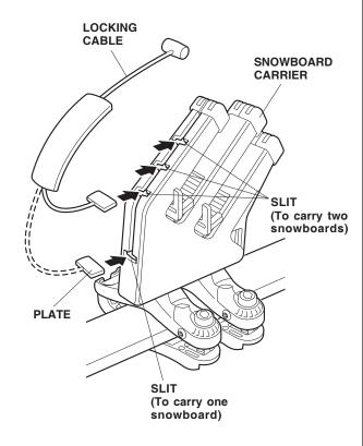
15. After loading the snowboard(s) on the carrier, adjust it (them) with the help of the board supports so that the top edges are level and the boards are as far down in the carrier as possible. To secure the snowboard(s) use the key to open the covers, and insert the locking cable stoppers into the holes in the carrier covers.
