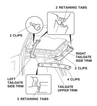
7. Remove the right and left tailgate side trims (one retaining tab and two clips).
