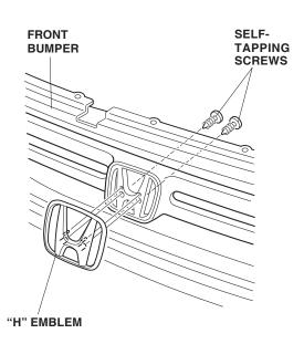
4. Attach the gold "H" emblem to the front bumper with the two self-tapping screws you removed.
