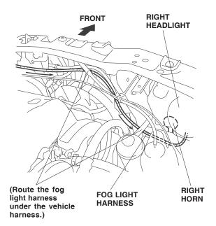
13. Secure the fog light harness to the vehicle harness with two wire ties.
