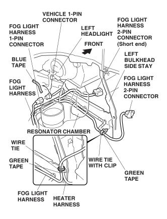
9. Route the other fog light harness 2-pin connector in front of the resonator chamber and secure the green tape on the fog light harness in close to the wire tie with clip to the hole in the left bulkhead side stay. If an engine block heater is installed, secure the fog light harness to the heater harness with one wire tie. 10. Secure the wire tie with clip to the hole in the left front bulkhead panel.
