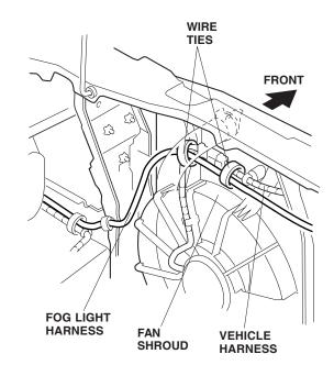
16. Above the right fan shroud, secure the fog light harness to the vehicle harness with five wire ties.
