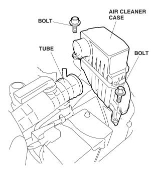
6. Remove the air cleaner case (2 bolts). Avoid damaging the vehicle harness in around of the air cleaner case, when removing the air cleaner case.
