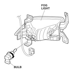
5. Reconnect the 2-pin connector, and reinstall the inner fender and clips.
