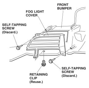
19. Install the left fog light on the front bumper using the retaining clip you removed and three 5 x 16 mm self-tapping screws.
