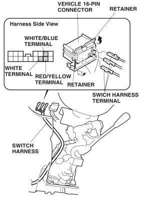
37. Slide the combination light switch onto the steering column and secure the combination light switch with the two screws removed in step 35. Hold the combination light switch case securely against the column while tightening the screws, do not push on the lever.
