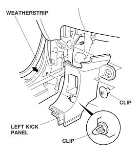
26. Remove the upper clip from the left kick panel, then pull the left kick panel out toward you to release the remaining clip.
