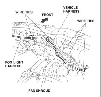
17. Below the right headlight, secure the fog light harness to the vehicle harness with two wire ties.
