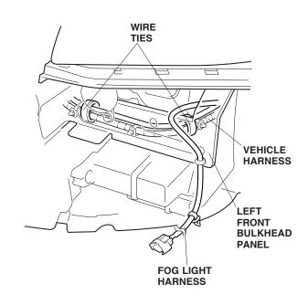
15. Above the left fan shroud, secure the fog light harness to the vehicle harness with two wire ties.
