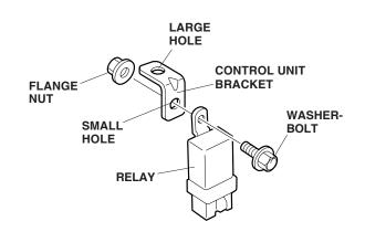
32. Plug the switch harness 4-pin connector into the relay.
