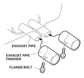
With the flange bolts facing down, slide the exhaust pipe finishers onto the exhaust pipes until they bottom. If necessary, use a rubber mallet to tap the exhaust pipe finishers into place.
