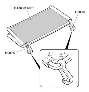
8. Attach the hooks to the anchors in the floor, and attach the loops to the tie-down hooks on the rear side trim panel.
