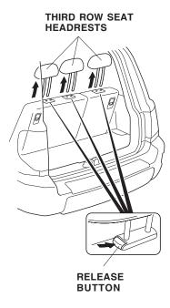
Store the headrests in the storage compartment under the cargo floor. Insert the posts of the headrests into the holes in the front of the storage compartment.
