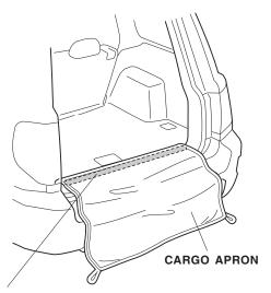
VELCRO STRIP (Align the Velcro strip on the cargo apron with the Velcro strip on the cargo liner.)
