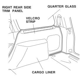
16. Remove the adhesive backing from the Velcro strip, fold the cargo liner over, and attach the strip to the right rear side trim panel. Press the Velcro strip firmly against the trim panel with the palm of your hand.
