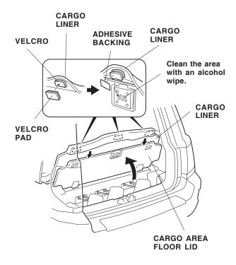
12. Remove the adhesive backing from each Velcro pad, and attach the Velcro pads to the storage compartment cover. Press the Velcro pads firmly against the cover with the palm of your hand.
