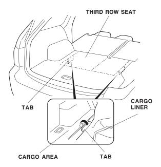
Open the cargo area floor lid, and fit the pocket of the cargo liner around the floor lid. Using one alcohol wipe, clean the area where the Velcro pads will attach.
