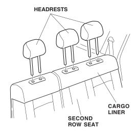
7. Install the cargo liner over the second row seat, then reinstall the headrests.
