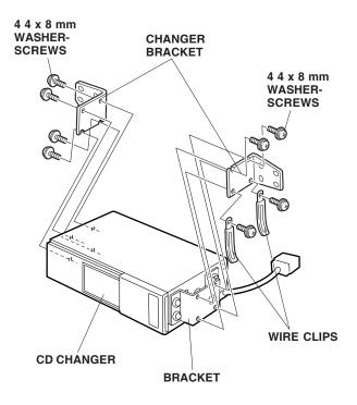
connector and secure the CD changer connector to the changer bracket with one wire tie with clip.
