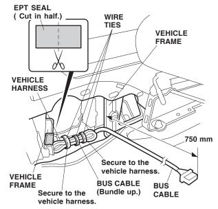
the vehicle frame. Bundle up the excess bus cable and secure it to the vehicle harness with three wire ties.
