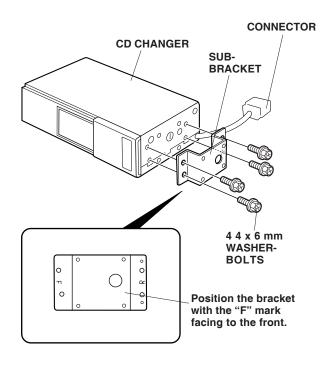
side of the CD changer with four 4 X 8 mm washer-screws. Attach two wire clips to the lower washer-screws. Install the changer bracket to other of the CD changer with four 4 x 8 mm washer-screws.
