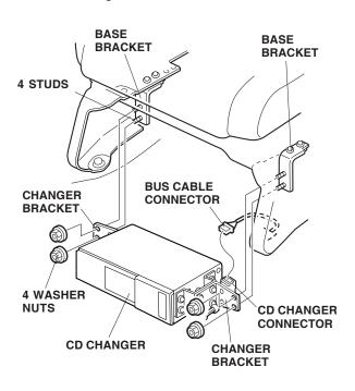
studs, and install the one washer nut on the end of each stud. Tighten the washer nuts securely.
