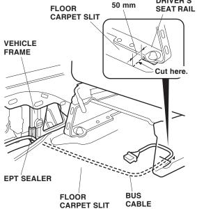
the area where the EPT sealer will attach. Attach half of an EPT sealer to the edge of the vehicle frame in the area shown.
