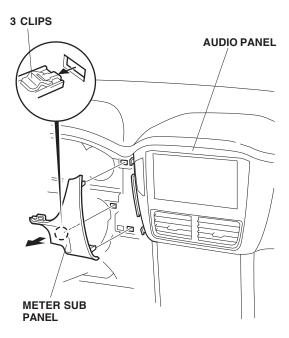
Gently pull out on the left side of the audio panel to release the remaining three clips.
