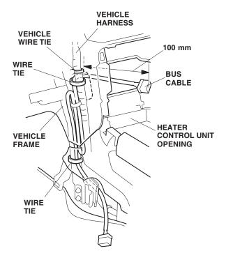
the driver's center console area, clean the vehicle frame where the EPT sealer will attach. Attach 1/2 of a cushion tape to the vehicle frame at the location shown.
