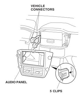
Remove the four screws that fasten the audio unit brackets. Pull the audio unit out toward you, ther unplug the vehicle connectors and vehicle antenna connector from the rear of the audio unit.
