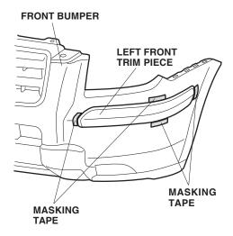
11. Attach a strip of masking tape to the ends of the four adhesive backings shown, and peel back 2 to 3 inches from the ends. Fold the ends up and tape them to the front of the trim piece. Remove the remaining two adhesive backings.
