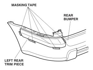
22. Attach a strip of masking tape to the ends of the adhesive backings shown and peel back 2 to 3 inches from the ends. Fold the ends up and tape them to the front of the trim piece. Remove the remaining adhesive backing.
