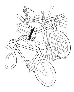
3. Tighten the bicycle arm straps securely around the bicycle frame.
