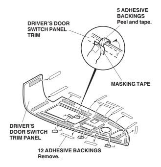
Peel one inch from the end of the five adhesive backings shown, and attach them to the front of the driver's door switch trim panel with masking tape. Remove all the remaining adhesive backings from the switch panel trim.
