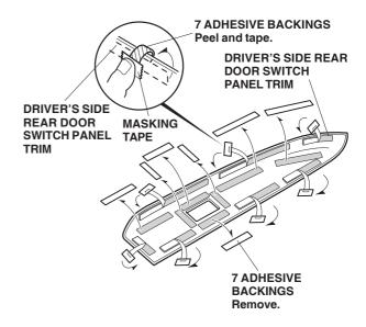
8. Peel one inch from the end of the seven adhesive backings shown, and attach them to the front of the driver's side rear door switch panel trim with masking tape. Remove all the remaining adhesive backings from the switch panel trim.
