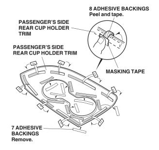
15. Peel one inch from the end of the eight outer adhesive backings shown, and attach them to the front of the passenger's side rear door cup holder trim with masking tape. Remove all the remaining inner adhesive backings from the cup holder trim.
