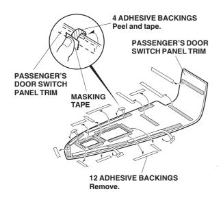
5. Peel one inch from the end of the four adhesive backings shown, and attach them to the front of the passenger's door switch panel trim with masking tape. Remove all the remaining adhesive backings from the switch panel trim.
