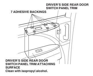
10. Repeat steps 7 thru 9 to install the passenger's side rear door switch panel trim to the passenger's side rear door switch panel.
