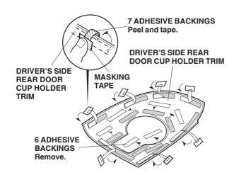
12. Peel one inch from the end of the seven outer adhesive backings shown, and attach them to the front of the driver's side rear door cup holder trim with masking tape. Remove all the remaining inner adhesive backings from the cup holder trim.
