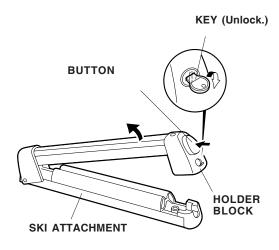
2. Position the skis on the attachment with the rear of the skis facing forward, and the bindings between the front and rear attachments.
