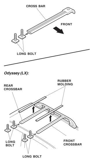
Reinstall the right side rail to the crossbars (if equipped), and torque the screws to 5 to 7 lb-ft (7 to 10 N·m). Reinstall the caps and crossbars (if equipped), and torque the TORX bolts to 7 lb-ft (10 N·m). Reinstall the roof rack cover (if equipped). 6. Insert the key, and turn it clockwise to unlock the front ski attachment. Press the button, and open the top frame completely.
