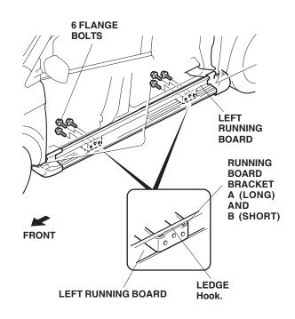
14. Tighten the 10 flange bolts and four flange nuts temporarily secured in steps 6 thru 8. Torque the flange bolts to 27 N·m (20 lb-ft).
