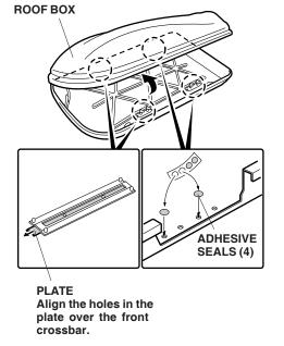
3. Attach an adhesive seal over the unsued rear mounting holes along the bottom of the roof box. The seal will help prevent water from entering the roof box. Remove the roof box from the vehicle.
