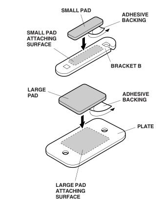
Using isopropyl alcohol on a shop towel, clean the four plates where the large pads will attach.
