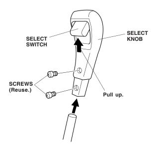
2. Get the new select knob from the kit and slide it onto the select rod while pulling up on the select switch in the direction shown.
