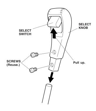
3. Reinstall the two screws.
