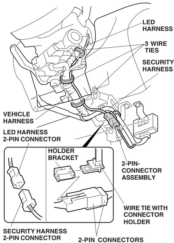
26. Plug the security harness 2-pin connector into the LED harness 2-pin connector.
