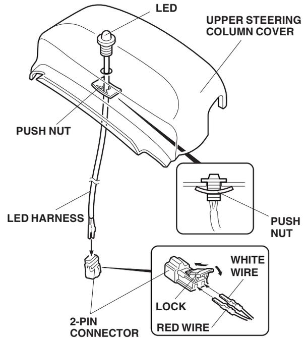
23. Get the 2-pin connector from the kit. Firmly push the LED terminals into the 2-pin connector as shown until they click. Secure the lock on the 2-pin connector.
