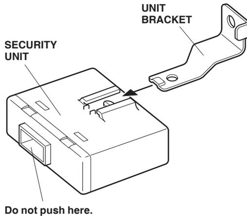
17. On the right of the steering shaft, remove the vehicle bolt and attach the security unit and bracket assembly using the vehicle bolt you just removed.
