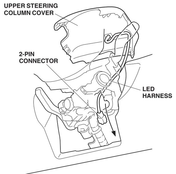
25. Secure the LED harness to the vehicle harness using three wire ties.
