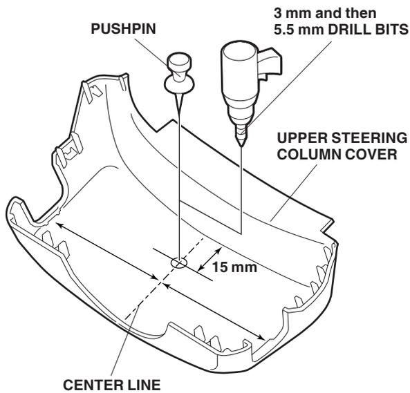
20. While wearing eye protection, drill a 5.5 mm hole at the pushpin mark. First drill with a 3 mm drill bit and finish with a 5.5 mm drill bit.
