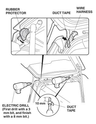
Temporary install the tailgate spoiler on the tailgate and insert the two bolts into the 8 mm holes. Using a felt-tip pen, mark the tailgate through the center hole in the tailgate spoiler. Remove the tailgate spoiler being careful not to drop the bolt on the vehicle.
