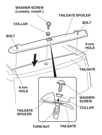
15. Position the tailgate spoiler on the tailgate and insert the two bolts into the 8 mm holes in the tailgate. Loosely install the washer-screw and the collar through the center hole in the tailgate spoiler and into the turn nut. Be careful not to drop the bolts on the vehicle. 16. Open the tailgate and install two cap nuts. Do not tighten the cap nuts yet.
