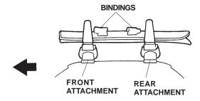
If the bindings cannot be positioned between the front and rear attachments, install the skis with one of the bindings positioned behind the rear attachment.
