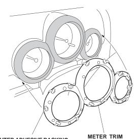
OUTER ADHESIVE BACKING (Peel back 2 to 3 cm (1/2 to 1 in.) from the end, and tape it to the front of the trim.)
