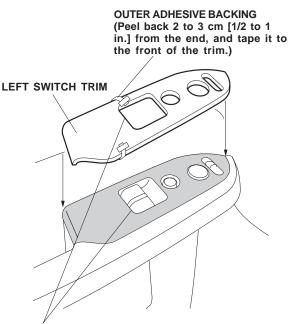
Check that the hole in the switch trim is aligned with the switch hole.
