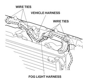
22. While holding the front bumper near the front of the vehicle, plug the fog light harness 2-pin connectors into the 2-pin connectors from the fog lights. Reinstall the front bumper.
