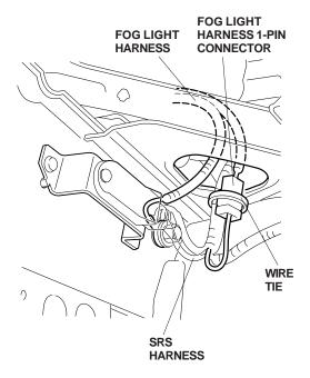
13. Behind the front side frame, route the fog light harness 2-pin connector (short end) down, and out through the clearance between the side frame and front bumper beam. Attach the wire tie with clip on the fog light harness into the hole in the side frame.
