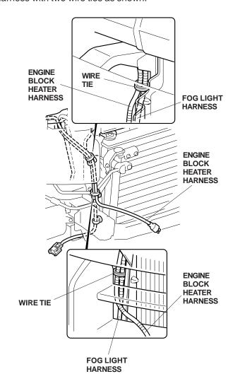
17. Secure the fog light harness to the hole with the wire tie as shown.
