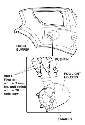
6. Using a hacksaw blade, cut out the marked area from the front bumper along the inside of the scribed line and the groove on the back. Remove all burrs from the edges of the cutout.
