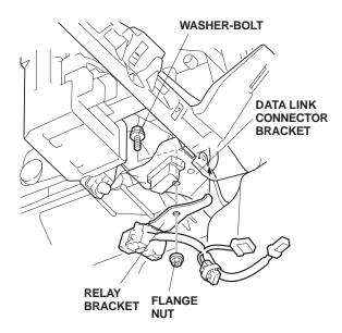
29. Locate the 3-pin connector blue-taped to the vehicle harness and remove the blue tape to free 3-pin connector. Slide the clip (supplied) onto the 3-pin connector you just freed.
