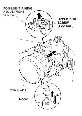
Remove the fog light connectors from the bracket stay, then unplug the connectors. Remove the fog light.
