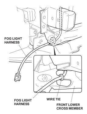
18. Secure the fog light harness to the holes in the bulkhead side stay and the left front bulkhead with the four wire ties with clip.
