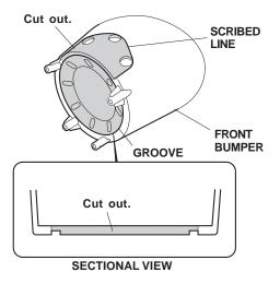
7. Inside the front bumper, slide the fog light into the cutout you made, and secure it with four self-tapping screws.
