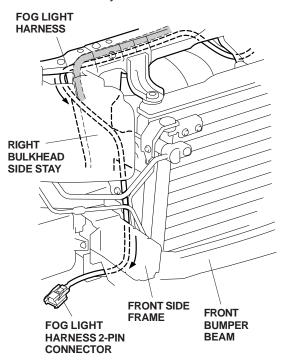
16. Attach the three wire ties with clip on the fog light harness into the holes in the bulkhead side stay. Further secure the fog light harness to the vehicle harness with two wire ties in the areas shown without engine block heater.
