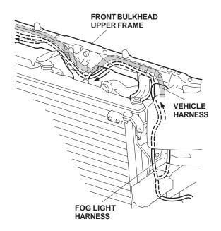
15. Continue routing the fog light harness 2-pin connector forward, then down to the bottom of the front side frame along the outside of the right bulkhead side stay.
