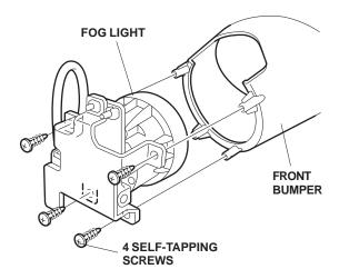
8. Repeat steps 5 thru 7 to cut the bumper and install the fog light on the right side of the bumper.
