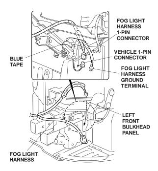
Locate the 1-pin connector blue-taped to the vehicle harness and remove the blue tape to free the 1-pin connector. Connect the 1-pin connector you just freed to the fog light harness 1-pin connector. 11. Remove the ground bolt that fastens the vehicle ground terminal and secure the fog light harness ground terminal using this ground bolt.
