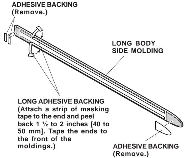
3. Using an alcohol wipe, thoroughly clean the areas where the long body side molding will attach.
