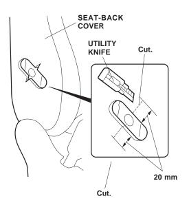
5. Using a felt-tip pen and tape measure, measure and mark the seat-back cover as shown. Push in on the mark, and confirm that the mark is centered over the hole in the seat base.
