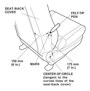
6. Using a utility knife, make two 70 mm (3 in.) cuts in the seat-back cover. Using these 70 mm (3 in.) cuts as a guide, cut out the seat urethane to expose the seat base.
