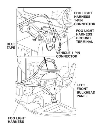
12. Locate the 1-pin connector blue-taped to the vehicle harness and remove the blue tape to free the 1-pin connector. Plug the 1-pin connector you just freed to the fog light harness 1-pin connector.
