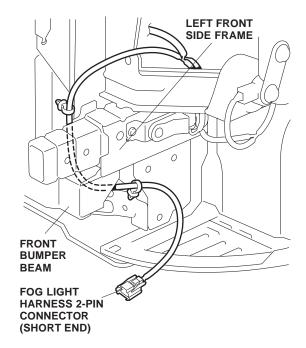
16. Route the fog light harness 2-pin connector (long end) from underneath the left headlight to the engine compartment, then along the vehicle harness behind the front bulkhead upper frame.
