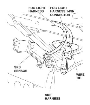
15. Behind the front side frame, route the fog light harness 2-pin connector (short end) down, and out through the clearance between the side frame and front bumper beam.
