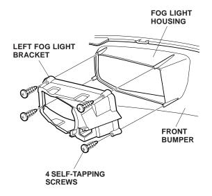
9. Insert the left fog light from the fog light opening at the front of the front bumper to the left fog light bracket and install it with one self-tapping washer-screw to the left fog light bracket.
