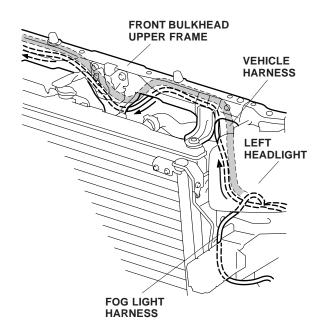
17. Continue routing the fog light harness 2-pin connector from underneath the right headlight to the front of the vehicle, then down to the bottom of the front side frame along the outside of the right bulkhead side stay.
