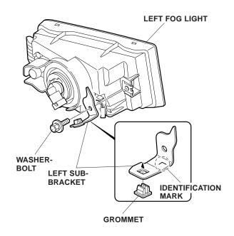
8. Inside the front bumper, slide the left fog light bracket into the cutout you made, and secure it with four self-tapping screws.
