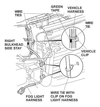
19. Secure the fog light harness to the vehicle harness with the eight wire ties in the areas shown.
