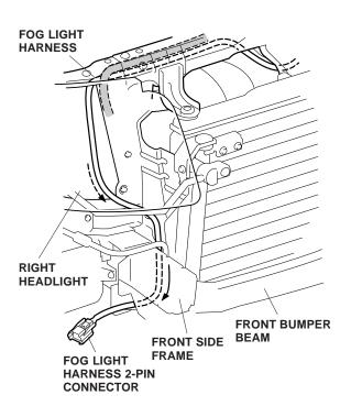
18. Push each of the two wire ties with clip on the fog light harness into the holes in the bulkhead side stay. Further secure the fog light harness to the vehicle harness with three wire ties in the areas shown.
