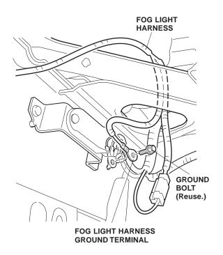
14. Secure the fog light harness 1-pin connector and the fog light harness to the vehicle harness with one wire tie. Do not secure the 1-pin connector to the SRS harness with the wire tie.
