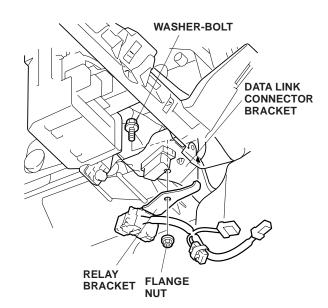
30. Locate the 3-pin connector blue-taped to the vehicle harness and remove the blue tape to free the 3-pin connector. Slide the clip onto the 3-pin connector you just freed.
