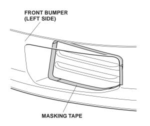
6. Inside the front bumper, locate the slit on the fog light housing on the left side. Using a utility knife, cut out the marked area from the front bumper along the groove on the back. Remove all burrs from the edges of the cutout.
