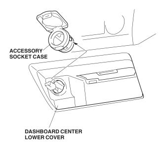
7. Slide the ring into the hole in the dashboard center lower cover in the direction shown.
