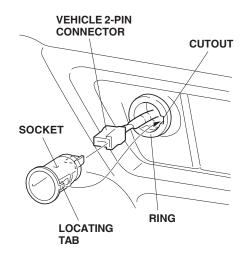
9. Align the locating tab on the socket with the cutout in the ring, and slide the socket into the ring.
