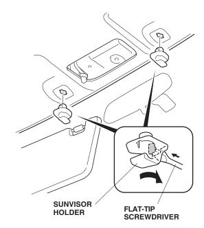
5. Remove the cap from the left sunvisor (four retaining tabs).
