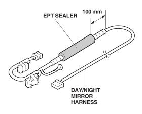
20. Tape a piece of steel wire to the 7-pin connector end of the day/night mirror harness. Pull the 7-pin connector up and out through the clearance between the left front pillar and the instrument panel.
