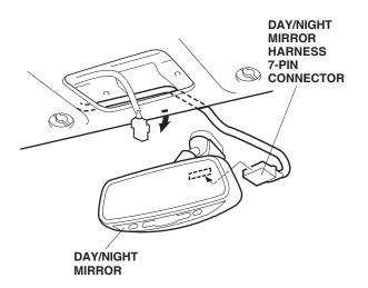
25. Measure the day/night mirror harness in the area shown. Route the day/night mirror harness through the grooves in the upper and lower covers. Attach the lower cover to the mirror stay. 27. Using isopropyl alcohol on a shop towel, clean the areas where the EPT sealer will attach. Under the roof liner, secure the day/night mirror harness to the roof panel with the four EPT sealers in the areas shown.
