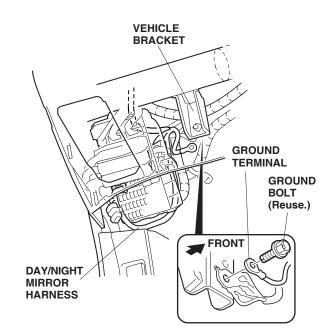
31. Secure the day/night mirror harness to the vehicle harness with four wire ties in the areas shown.
