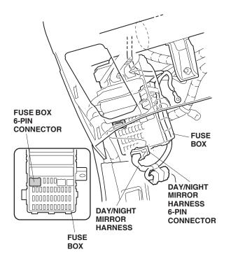
NOTE: If another accessory is already plugged into the 6-pin connector, remove the dummy connector from the 6-pin connector taped to the day/night mirror harness. Disconnect the 6-pin connector of the other accessory harness from the fuse box and connect it to this 6-pin connector.
