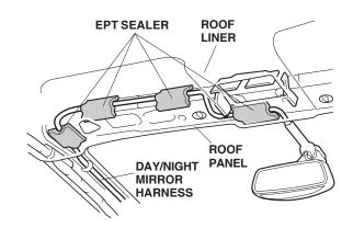
28. Secure the day/night mirror harness to the vehicle harness with three wire ties in the areas shown.
