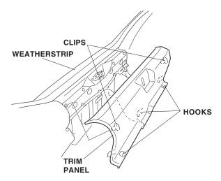
Remove the clips, and then remove the left trunk side trim panel from the trunk. Release the rear seat-back release cable out through the slit in the trim panel.
