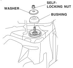
36. Torque the damper shaft self-locking nut to 29 N·m (21 lb-ft) while holding the damper shaft with a hex wrench.
