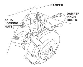
11. Install the wheel sensor harness clip and the brake hose bracket to the damper.
