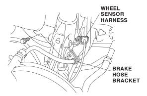
Remove the damper pinch bolts and self-locking nuts from the damper. Do not allow the knuckle to rotate too far outward. This may allow the inner CV joint bearing to unseat.
