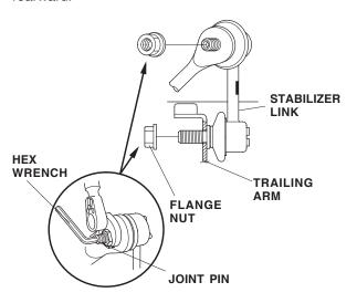
34. Install the stabilizer link on the trailing arm with a new self-locking nut, and lightly tighten both nuts.
