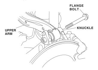
32. Install the damper mounting bushing onto the damper unit, and install the damper unit. Slowly raise the jack until you can align the bolt hole with the holes in the trailing arm and the damper, and then install the new flange bolt.
