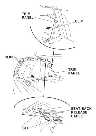
Remove the right trunk side trim panel the same way. 18. Position the floor jack at the connecting point of the trailing arm and the knuckle. Raise the floor jack until the suspension begins to compress. Remove the flange bolt from the bottom of the damper.
