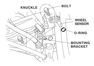
20. Remove the brake hose mounting bracket. Using needle nose pliers, disconnect the wheel sensor clip from the brake hose mounting bracket.
