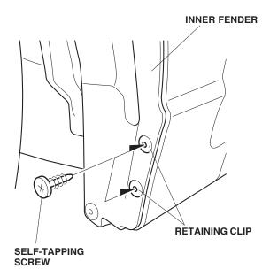
18. Using a self-tapping screw, pierce a hole through the center of the inner fender retaining clips.
