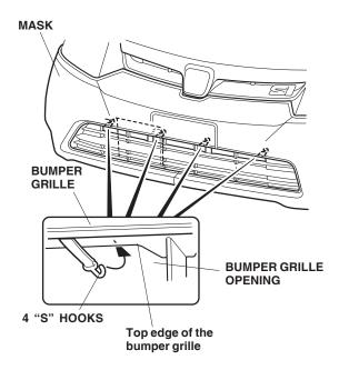
17. Attach the four "S" hooks to the bottom inside edge of the bumper grille opening.
