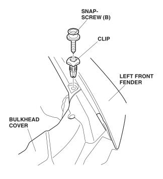
4. Repeat steps 2 and 3 to install a snap-screw (B) on the right side of the vehicle.
