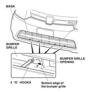
18. Route the elastic cord through the 10 loops on the bottom of the mask. Attach one "S" hook to the bottom edge of the bumper on one side. Stretch out the cord after routing it through each loop, then attach the other "S" hook to the bottom edge of the bumper on the other side.
