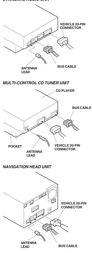
43. Connect the four vehicle connectors to the center panel, and reinstall the center panel.
