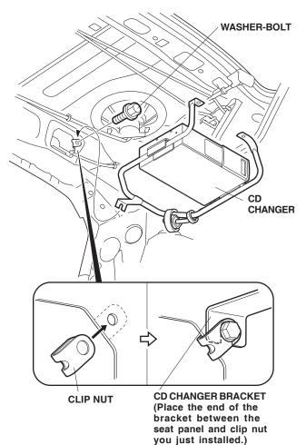
39. Slide the two clip nuts onto the CD changer brackets and parcel shelf through the holes in the parcel shelf, and align their holes as shown. Install the two washer-bolts, and tighten them securely.
