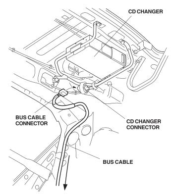
41. Fold the excess bus cable, and secure it to the holes of the rear seat panel with the two wire ties with clip.
