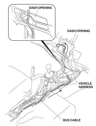
25. Measure 300 mm from the end of the bus cable connector, then secure the bus cable to the vehicle harness with three wire ties.
