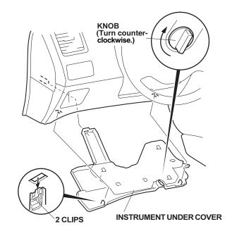
14. Release the eight clips, and remove the instrument lower cover by pulling it towards you. Take care not to damage the clips.
