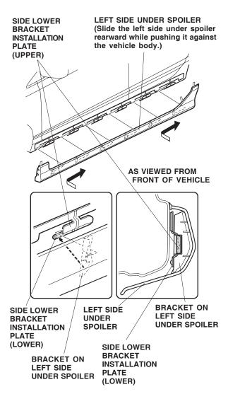
20. Check that all six brackets of the left side under spoiler are set in the side lower bracket installation plates.
