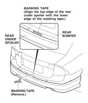
14. While applying pressure on the rear under spoiler, carefully remove the adhesive backings in the sequence shown. After removing, hold the rear under spoiler firmly against the rear bumper with the palm of your hand for 30 seconds.
