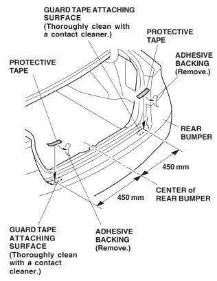
Remove the adhesive backing from each of the protective tapes, and attach the tapes to the rear bumper as shown.
