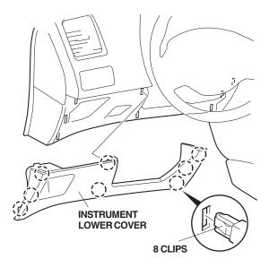
15. Release the four clips, and remove the assistant lower cover by pulling it toward you. Take care not to damage the clips and pins.
