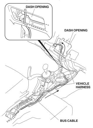
25. Measure 300 mm from the end of the bus cable connector, then secure the bus cable to the vehicle harness with three wire ties.
