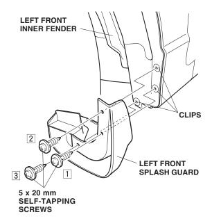
4. Turn the steering wheel all the way clockwise, and repeat steps 2 and 3 to install the right front splash guard.
