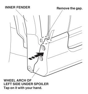
25. Loosely install the front self-tapping screws in the holes in the wheel arch of the left side under spoiler.
