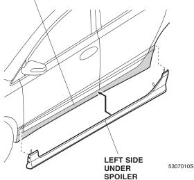
2. Using a tape measure and felt-tip pen, measure and mark the body area shown.
