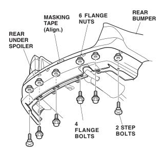
13. Check that the top edge of the rear under spoiler aligns with the lower edge of the masking tape you attached in step 1, and remove the masking tape.
