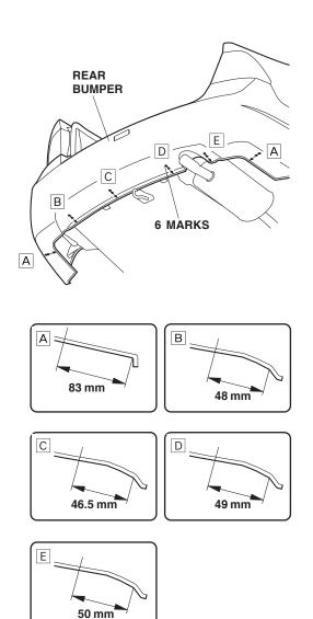
9. Using a pushpin, make a hole through each marked location on the rear bumper.
