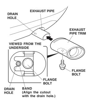
2. Slide the exhaust pipe trim onto the exhaust pipe until it bottoms against the exhaust pipe.
