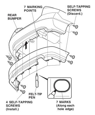
While holding pressure on the rear under spoiler, use a felt-tip pen to mark the rear bumper along each hole edge in the bracket on the rear under spoiler. NOTE: If a gap is visible between the rear bumper and under spoiler, remove the rear under spoiler and measure the centerline distance to the edge of the rear bumper and mark as shown.
