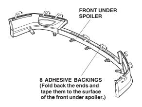
8. Using isopropyl alcohol on a shop towel, clean the front bumper where the front under spoiler will attach.
