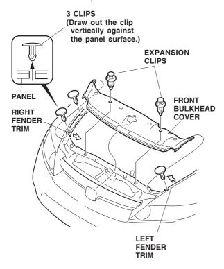
Remove the front bumper (two bolts, ten clips, and two self-tapping screws and pull the bumper out towards you). If equipped, unplug the fog light connectors. If equipped, unplug the front corner sensor connectors. Place the front bumper on a blanket to install the front under spoiler.
