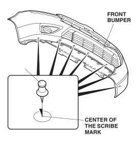
4. Using a drill, drill a 10 mm hole through each marked location from the front of the bumper. First drill with a 3 mm bit, and finish with a 10 mm bit. Remove any burrs from the edges of the holes with a file.
