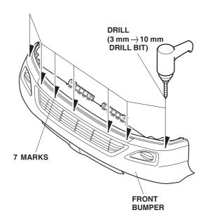
Using a drill, drill a 3 mm hole through four dimpled areas of the front bumper on both sides. Remove any burrs from the edges of the holes with a file.
