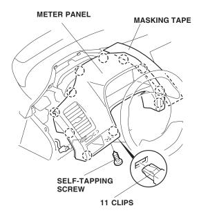
9. Apply masking tape to the instrument panel as shown, and remove the center panel (two bolts, ten retaining clips, and unplug the vehicle connectors).
