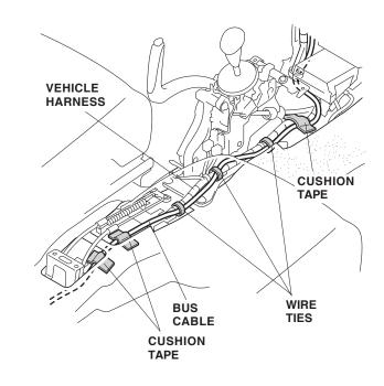
25. Using isopropyl alcohol on a shop towel, clean the areas where the cushion tape will attach. Attach the bus cable to the floor panel with the three cushion tapes in the area shown.
