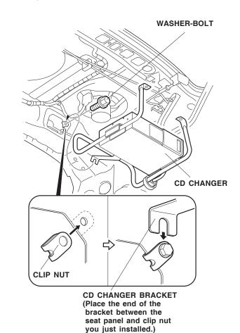
35. Loosely install the washer-bolt to the rear seat panel first. Then, place the end of the CD changer bracket between the seat panel and clip nut you just installed.
