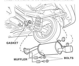
Torque the bolts to 22 N·m (16 lb-ft), alternating from side to side.
