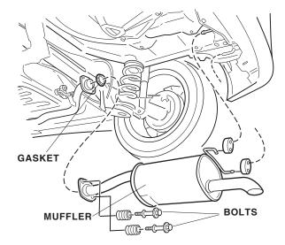
Remove the old exhaust gasket, and replace it with the new exhaust gasket from the kit.
