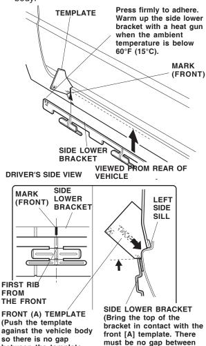
12. Press the front end of the side lower bracket (where you removed the adhesive backing) to adhere the part firmly to the vehicle body.
