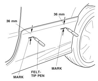
37. Using isopropyl alcohol on a shop towel, attach the sticker to the side under spoiler at the marks you made in step 36. Align the corner of the sticker to the rear edge of the side under spoiler.
