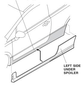
2. Using a tape measure and felt-tip pen, measure and mark the body as shown.
