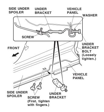
30. Position the under bracket on the side under spoiler, and loosely install the two screws. Tighten the under bracket bolt, but don't tighten it completely yet. 31. Align the rear top edge of the left side under spoiler with the edge of the radius of the vehicle panel as shown. Remove the five adhesive tapes from the left side under spoiler. Press firmly on the side under spoiler.
