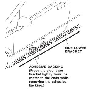
When the ambient temperature is below 60°F (15°C), warm up the entire side lower bracket to 60°F (15°C) or above before attaching it to the vehicle body.
