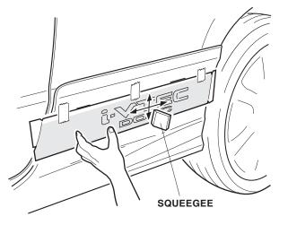
40. Gently peel off the protective film at an angle.
