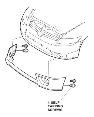
6. While applying pressure to the front under spoiler, carefully remove the adhesive backings in the sequence shown. After removing, hold the front under spoiler firmly against the front bumper with the palm of your hand for 30 seconds. Tighten the self-tapping screws installed in step 5.
